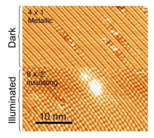
Fig. 1. Optical control of transition from  $4 \times 1$  metallic (upper area) to  $4 \times 1$  insulating (lower area) phases.
